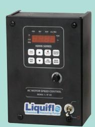
Plug And Play And You're On Your Way the box and plug into a 115 VAC wall outlet. The VFD allows the motor speed, thus the pump flow rate to be manually controlled via the keypad or potentiometer. The digital display can be easily configured to read frequency (Hz), RPM or 0-100%.
